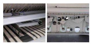
The first cross fold has an effective opening of 900 mm, which allows 3400 mm parts to be folded by making 2 lengthways folds.
