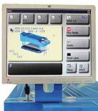
Monitor application for machine status display. Client/item in production, program, production data.
