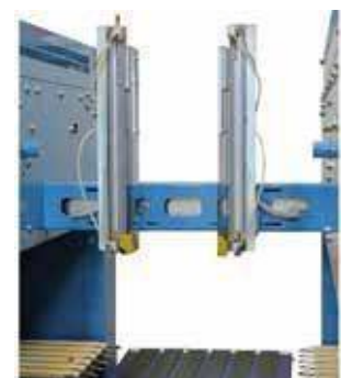
Anti-tip device for twinned machines.
