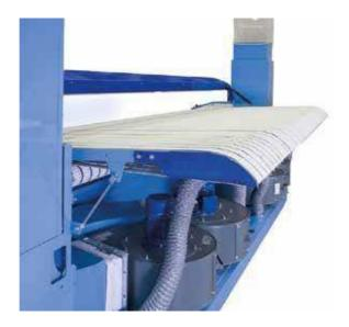
**Direct introduction** provides a wide suction surface to maximise control of the item as it is fed into the flatwork ironer.
