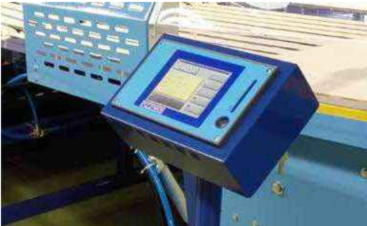
Touch screen Mavis management and adjustment terminal Single screen for managing up to six machines
