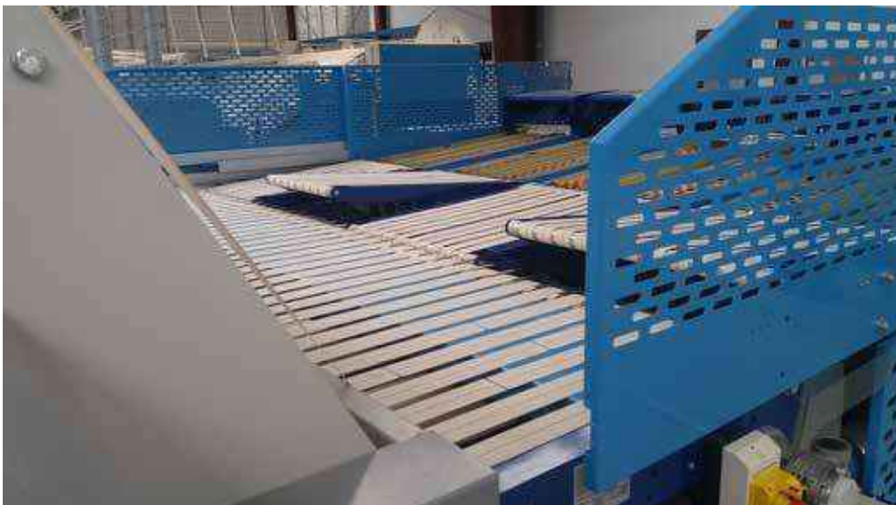
Movable cover during feed-in process - to avoid jams in the folding machine. Option of using the system as broken/dirty
